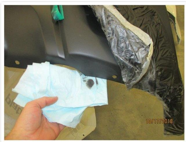
Further proof to this, the tape I pulled back on the textured part peeled some of the primer off the bumper cover
