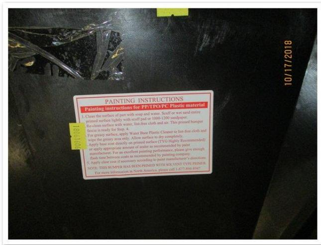
Conclusion: This bumper does not adhere to OEM quality standards, as this primer will fade over time exposing the poor nature of the primer used over the surfaces that are supposed to be raw plastic. Primer Degradation is to be expected with a product of this nature, it is unacceptable to send a vehicle out with raw primer exposed and call it pre-accident condition, this is an unfit repair.
